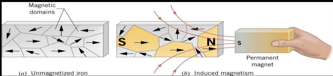
Dropping or banging a permanent magnet can disalign the magnetic domains and thus have a weaker B-field.
