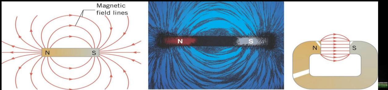
Picture notes: a) Magnetic field lines; b) magnetic field lines made with iron filings; c) magnetic field lines – constant between poles.
