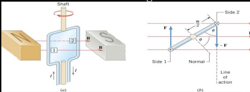
The normal is perpendicular to the plane of the loop
