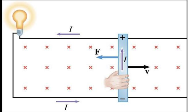
If the force went with the motion of the rod, then it would accelerate without bound.
